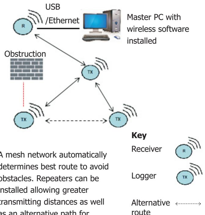
A mesh network automatically determines best route to avoid obstacles. Repeaters can be installed allowing greater transmitting distances as well as an alternative path for information to be relayed. In result, a robust network can be formed.
