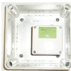
Transmitter in protective housing
